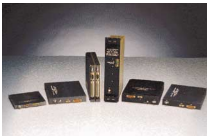
1. Typical digital frequency discriminators (DFDs) come in many form factors depending upon required frequency range and application.
