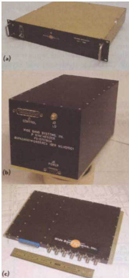
▲ Fig. 1 The synthesizer's three physical configurations: the 2U rack chassis (a), the replacement package (b) and the integrated package (c).
